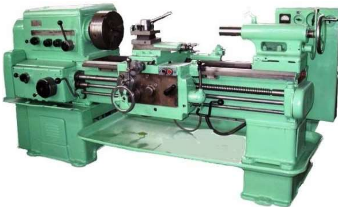
15.1-rasm. 1K62 modeli universal tokarlik vint-kesar dastgohining asl haqiqiy ko'rinishi.
